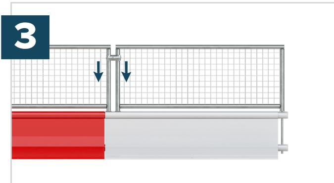
The pedestrian and vis rails/guards slot neatly into the top of the barriers and no additional pins are needed.
