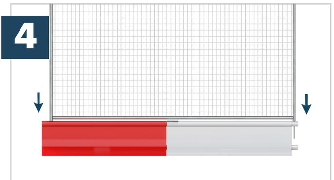
With the connecting pin in place, you can then insert the fence panel in to either end of the barriers.
