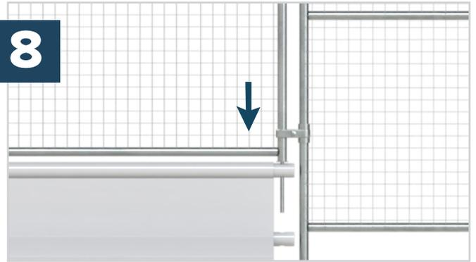
Slot the mesh fence panels into the top of the manta barriers.
