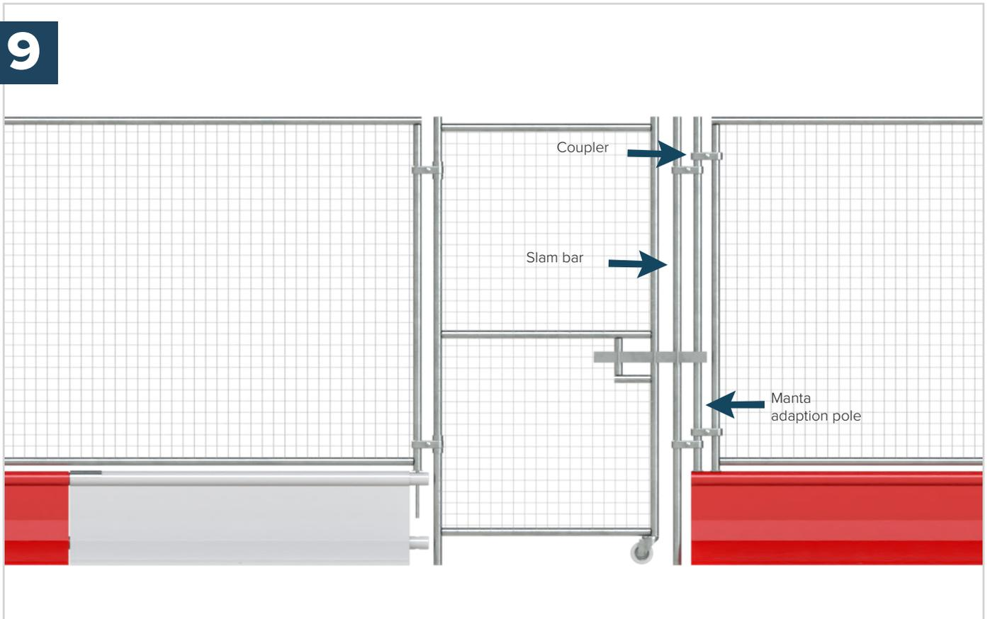
A gate hinge connects a gate to the fence panel. The pedestrian gate is then hung from the fence panel using an adaption pole and slam bar.
