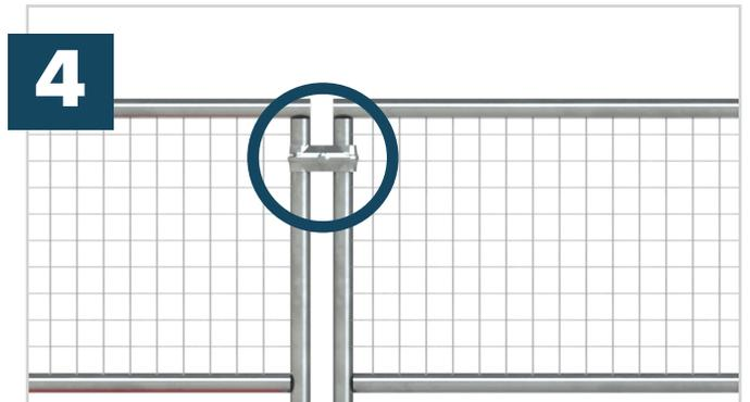
Secure the panels in place using a standard coupler.
